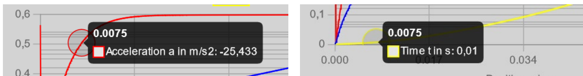
Figure 9 Point of deceleration = 2.5g at buffer shock at lower car speed with minimum load
