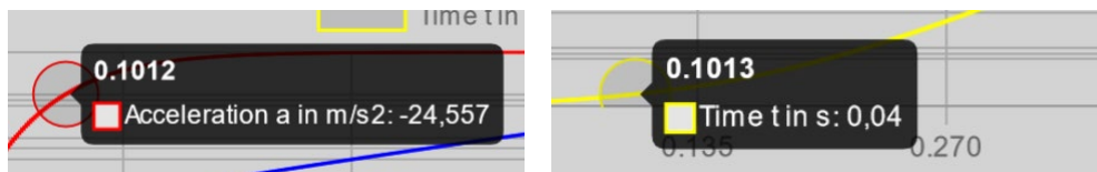
Figure 17 Point of deceleration = 2.5g at modified buffer shock at higher car speed with minimum load
