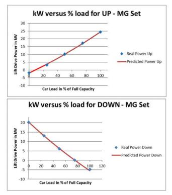
Figure 3(c) Power Curves of a typical M-G Set Drive
