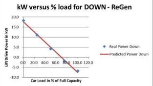
Figure 3(b) Power Curves of the same ACVVVF Drive with re-generative braking For ACVVVF drive without re - generative braking :
