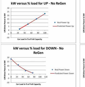
Figure 3(a) Power Curves of an ACVVVF Drive without regenerative braking
