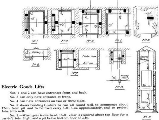
No. 7.—When gear is required below, a room may be set at the side of lift
