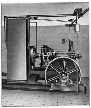
Electric Lift Winding Engine.
