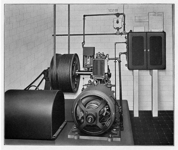
Winding Engine in basement.
